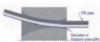
PE pipe through bell-mouth deviator, from anchorage to anchorage (most common detail)
