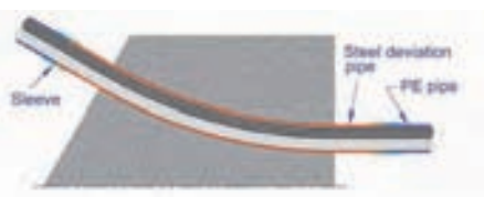
Deviation pipe protrudes from concrete at sufficient distance and is coupled to PE pipe
